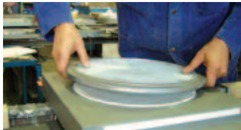
Above: Assembly of a spherical bearing Below: Pot bearing in accordance with EN 1337 and also with German U-label approval
