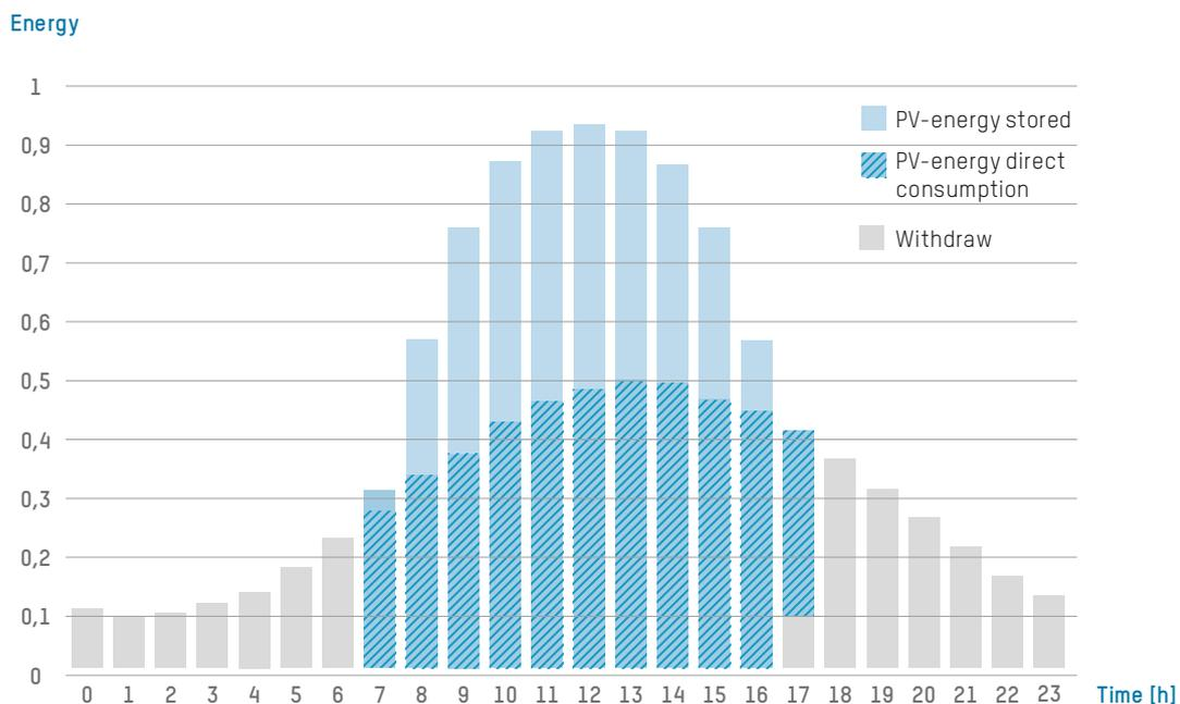
Example of the continuous energy supply with a large PV system and a Gravity Storage plant of suitable diameter.
