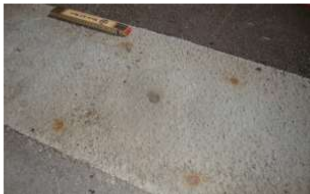
Testing of penetration of a point load (long bar at center). On right, deformation has fully reversed.
