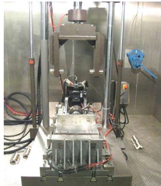
Movement testing at -40° to +60°C
