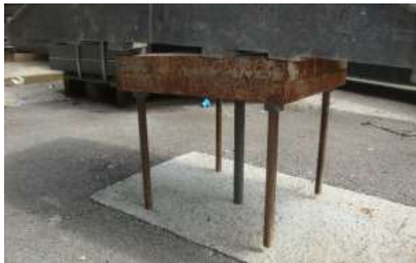
Testing of penetration of a point load (long bar at center). On right, deformation has fully reversed.
