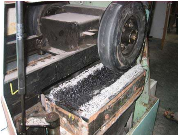
Comparison of common asphaltic plug joint material and the new Polyflex®Advanced flexible plug joint material after rutting test acc. to EN 12697-22 at 60°C (Left: Common asphalt plug material after 100 cycles at 60°C. Right: Polyflex®Advanced after 30,000 cycles at 60°)
