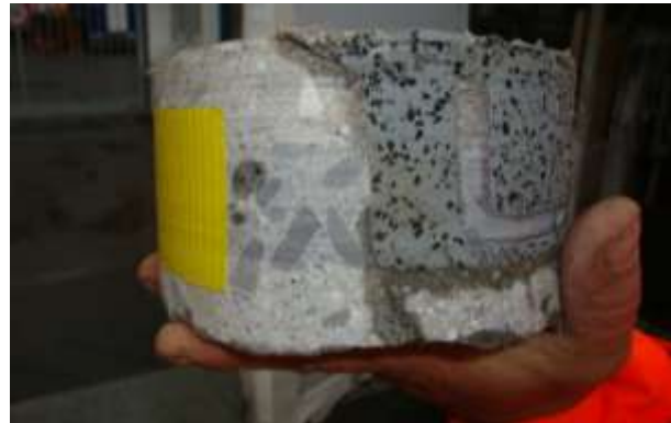
Core showing solid bonding to structure concrete
