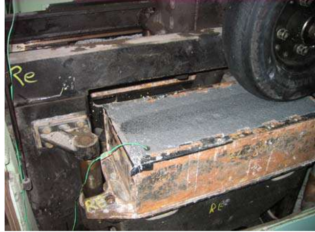
Comparison of common asphaltic plug joint material and the new Polyflex®Advanced flexible plug joint material after rutting test acc. to EN 12697-22 at 60°C (Left: Common asphalt plug material after 100 cycles at 60°C. Right: Polyflex®Advanced after 30,000 cycles at 60°)
