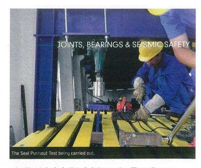
cycles with a velocity of 1m/s, with longitudinal movements or 450mm and transverse movements of  $\pm 250$ mm arising, and with rotations about every axis. These factors varied for the other tests, allowing the performance of the joint during a range of seismic events to be assessed.
