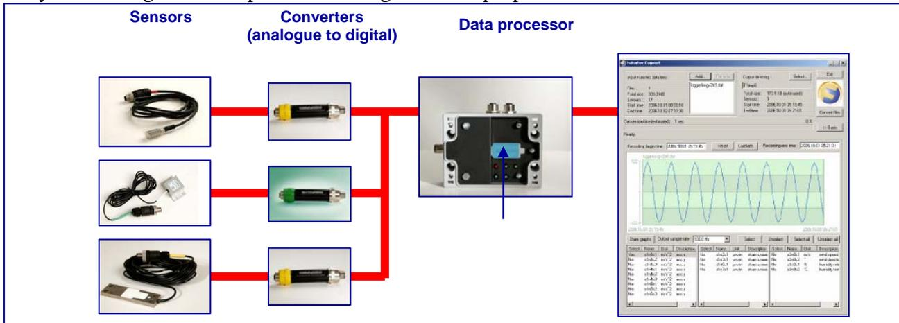
Fig. 6 Configuration of proposed system
