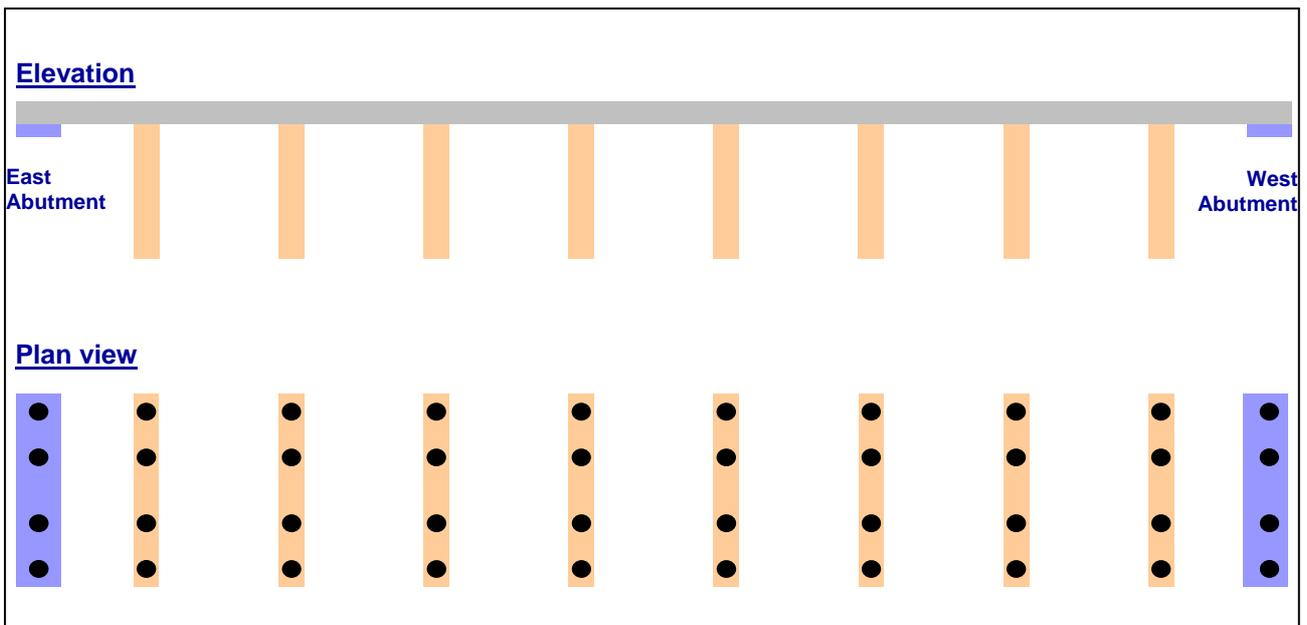
Fig. 3 Schematic layout of the bridge
