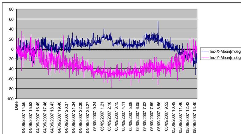
Fig. 10 *Inclination (used to measure rotation in two directions at one sensor location)*
