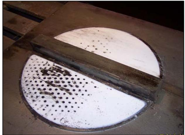
Fig. 2 Damage to PTFE of bridge bearings
