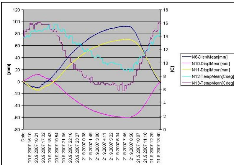
Fig. 11 Correlation between longitudinal displacement and temperature at one location
