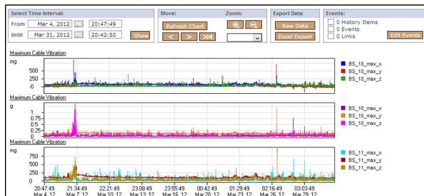
Figure 2. Example of display of recorded data (vibrations in three stay cables)
