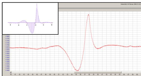
Figure 11. Crack widths (main graph), demonstrating excellent correlation with calculated influence line of static model for non-cracked condition (inset graph)
