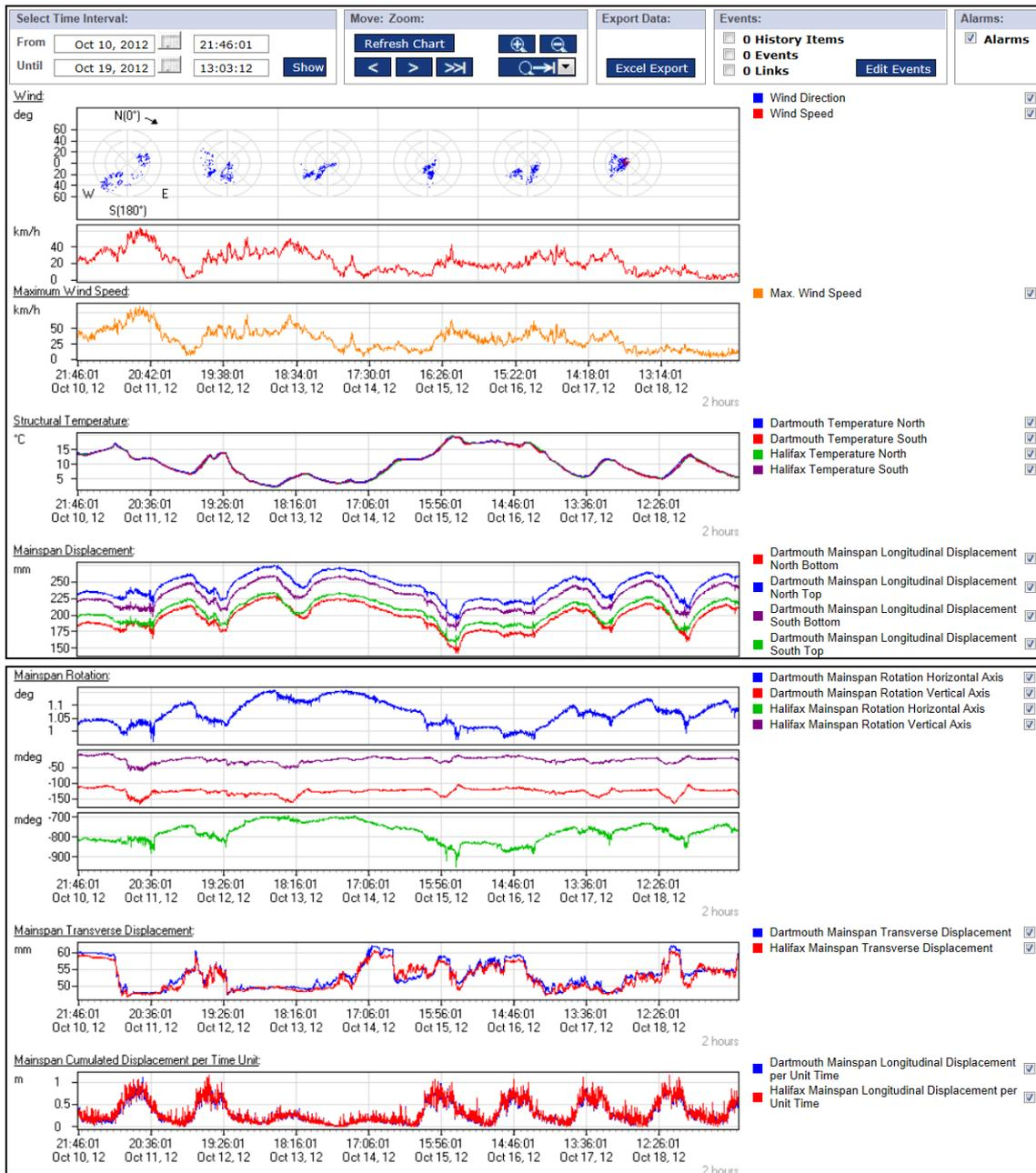
Figure 14. Example of data recorded by the monitoring system of the Angus L. Macdonald Bridge during a selected 9-day period. Rotations and displacements (both longitudinal and transverse) can be easily related to temperature, and to wind strength and direction
