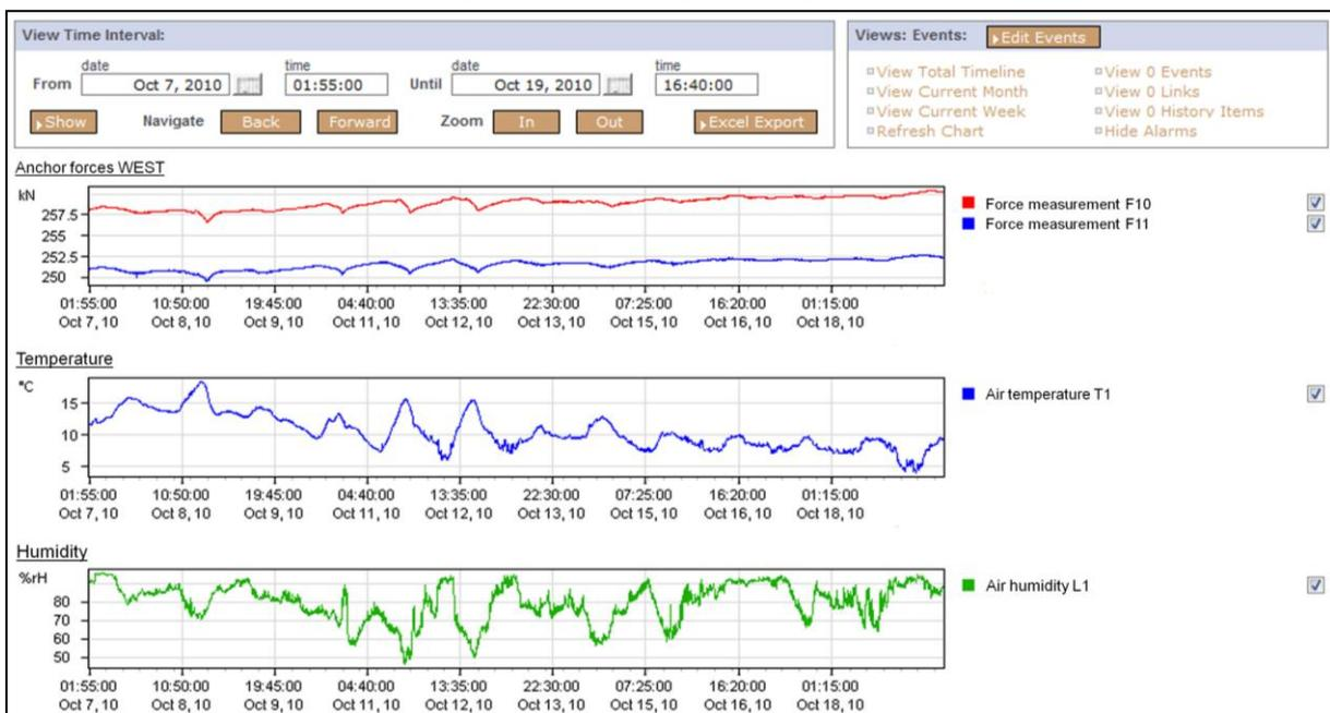
Figure 5. Graphical presentation of measured data relating to two specific anchors
