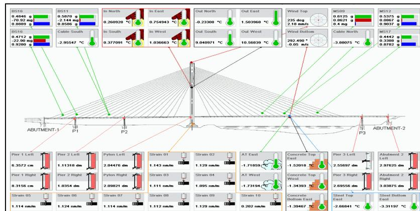
Figure 1. The "Cockpit" of the SHM system's user interface – presenting the current values of all main variables for an immediate overview
