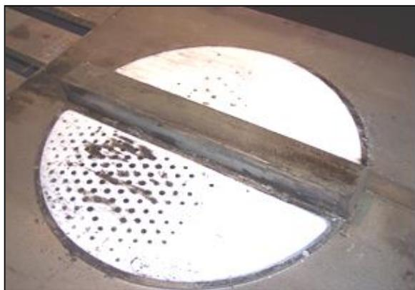
Figure 8. Wear of PTFE sliding discs
