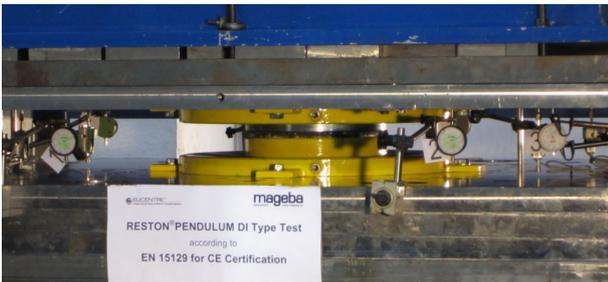
Figure 14. Testing of a curved surface slider per EN 15129. Four isolators were subjected to a total of 64 tests with 192 cycles, with vertical loads of -8000 kN to +1150 kN, and displacements of up to +/- 259 mm at velocities of up to 275 mm/s
