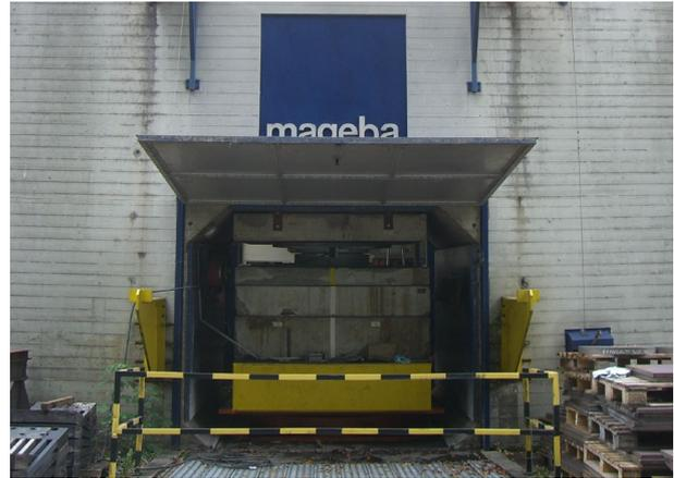
*Figure 9. A large bearing test rig with a vertical capacity of 100,000 kN (external view)*
