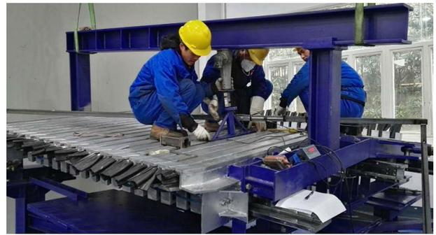
Figure 4. *Seal Push-Out Test*
