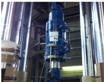
Figure 17. Prototype damper during testing at Politecnico di Milano, Italy
