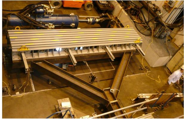
Figure 6. Seismic testing of a 7-gap modular joint at ATLSS Center, Lehigh University, PA, USA
