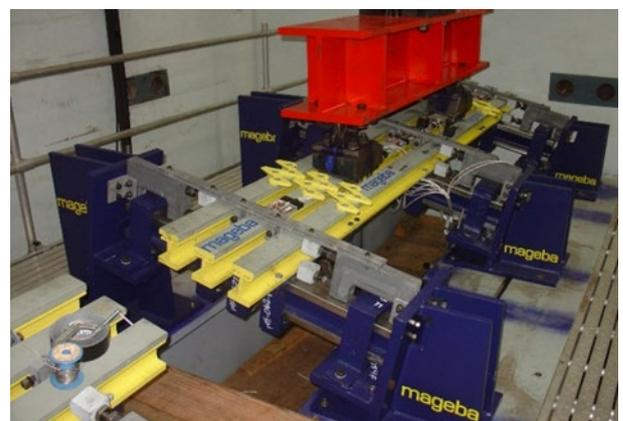
Figure 5. *Fatigue testing of Tensa-Modular joint*
