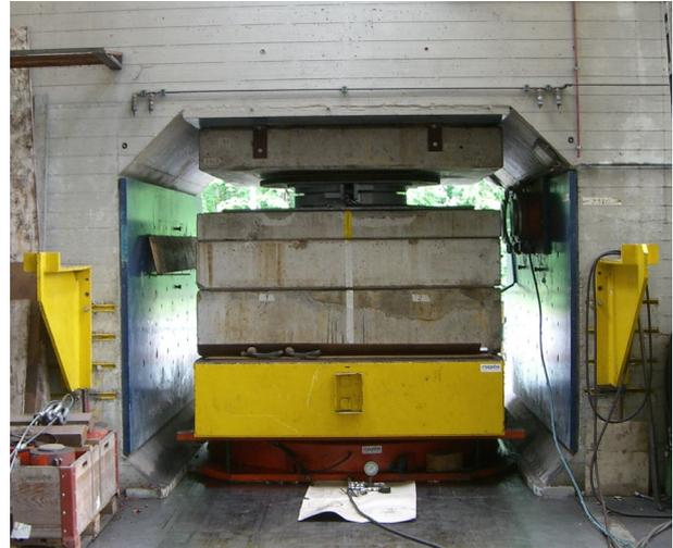
*Figure 10. Internal view of the test rig shown in Figure 9, showing ability to apply transverse forces or allow movements*
