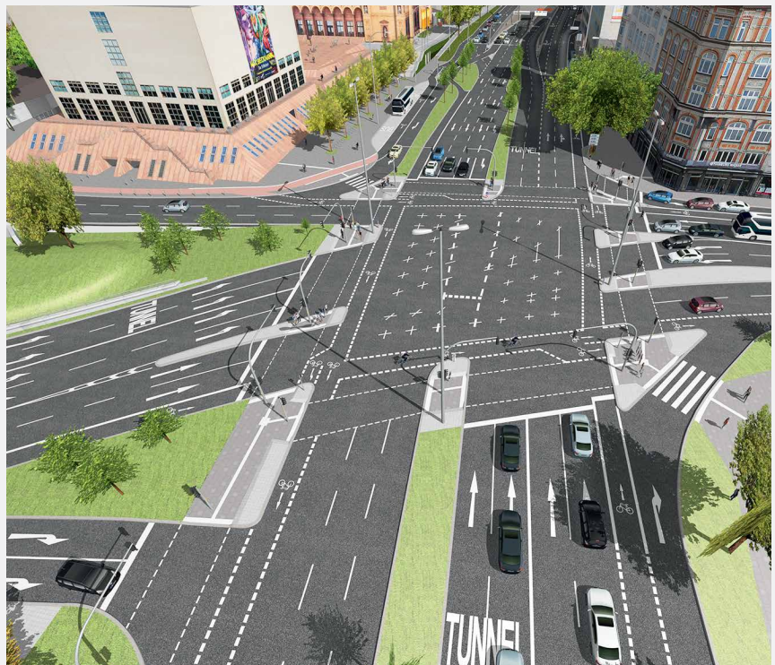
Complex traffic signals control, re-design of Ferdinandstor junction, Hamburg
