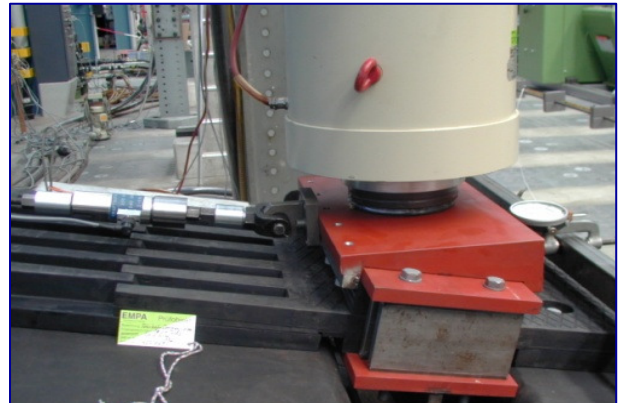
Fig. 15: Laboratory testing of a Tensa® Flex RC sliding finger expansion joint – with 2 million load cycles of 128 KN each
