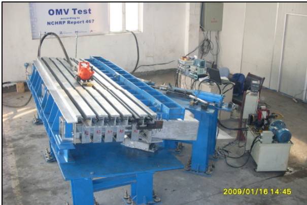
Fig. 14: Laboratory testing of a Tensa® Modular expansion joint – an Opening Movement Vibration (OMV) Test
