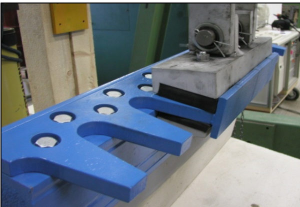
Fig. 13: Testing of Tensa® Finger Type RSFD cantilever finger joint, with two million load cycles
