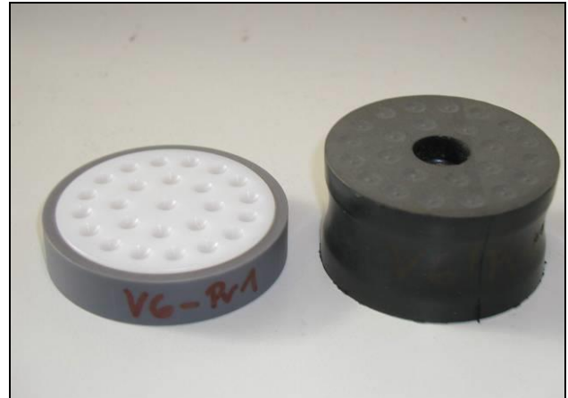
Figure 3 – A sliding bearing and a sliding spring of a modern modular expansion joint – used as a pair (above and below beam) to control the position of a centerbeam or support bar while allowing it to slide
