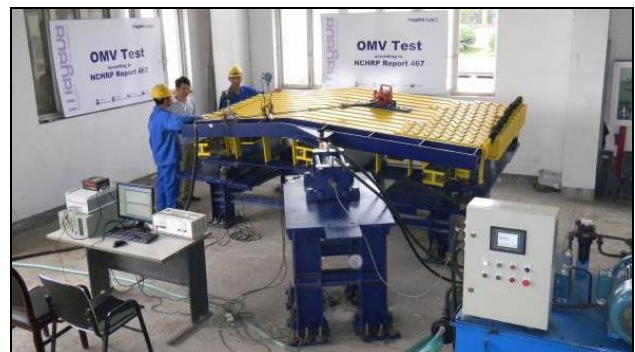
Figure 7 - Opening Movement Vibration (OMV) Test per NCHRP Report 467
