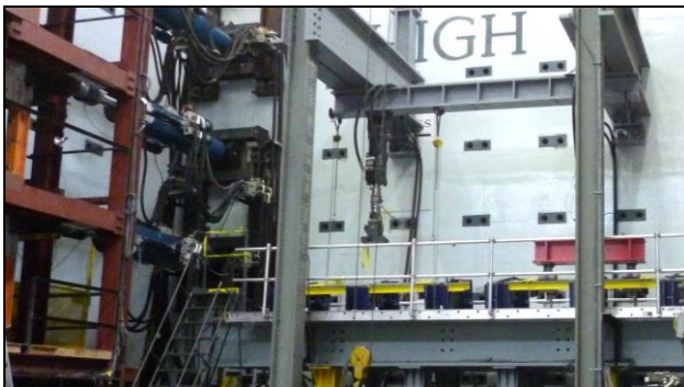
Figure 6 - Fatigue testing of joints (yellow) per NCHRP Report 402
