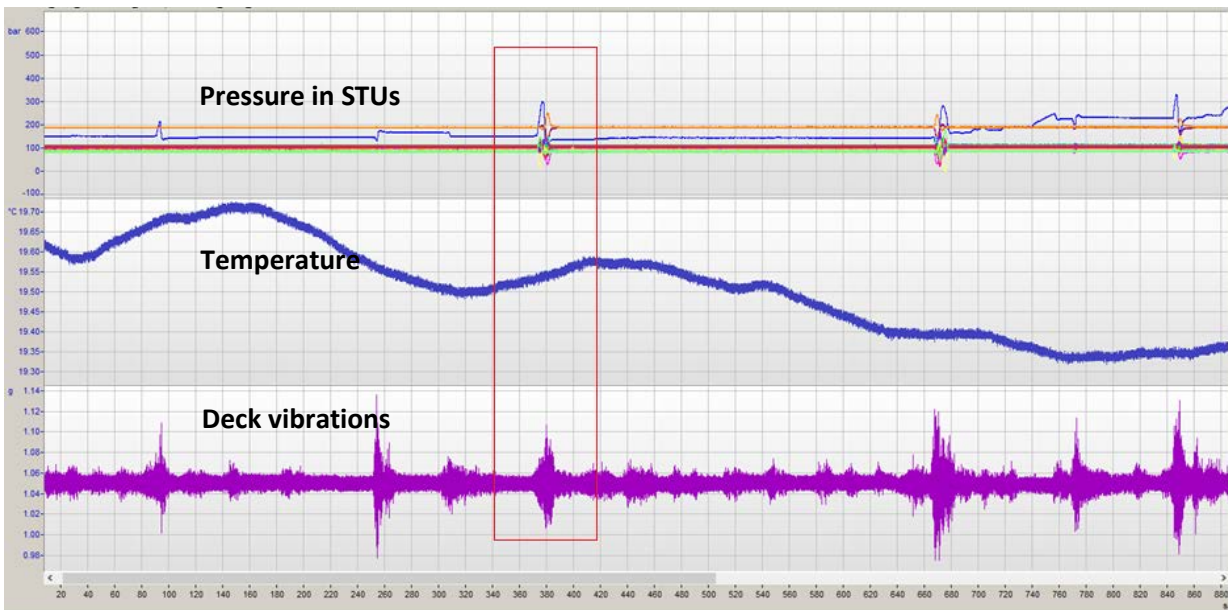
Figure 13. 100 Hz data measurements showing influence of traffic (indicated by deck vibrations) on STUs
