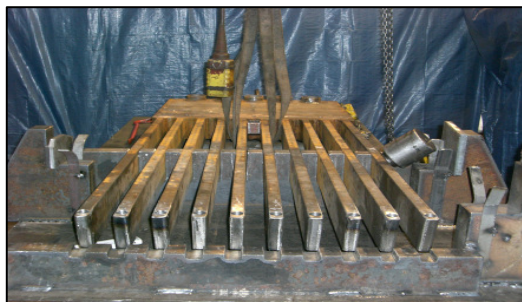
Figure 9. Mechanical straightening of the fingers of a sliding finger plate.
