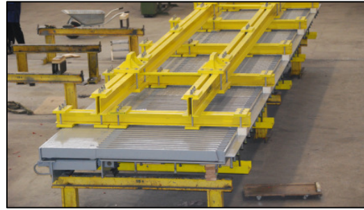
Figure 12. A sliding finger joint in the factory, with transportation frame (yellow).
