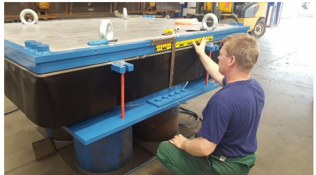
Figure 17. This guided-sliding bearing, shown here with protective dust skirt around edge and transportation fixings, was designed for a vertical load of 98,000 kN (approx. the weight of the Eiffel Tower) while accommodating longitudinal sliding movements of +/- 250 mm
