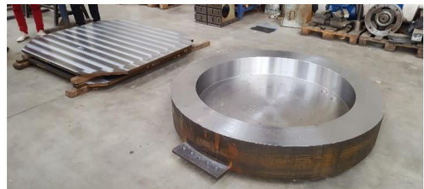
Figure 10. Early stage in the production of a large free-sliding pot bearing, with holes etc. as required for pressure sensors and injection process
