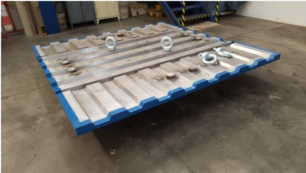
Figure 21. The guided-sliding bearing shown in Figures 19 and 20, as fabricated
