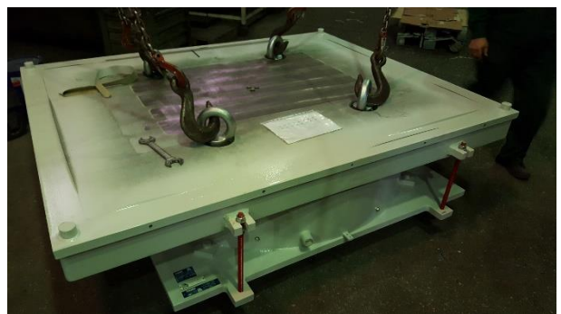
Figure 18. This free-sliding bearing was designed for a vertical load of 119,000 kN and to accommodate sliding movements of +/- 250 mm (longitudinal) and +/- 30 mm (transverse)
