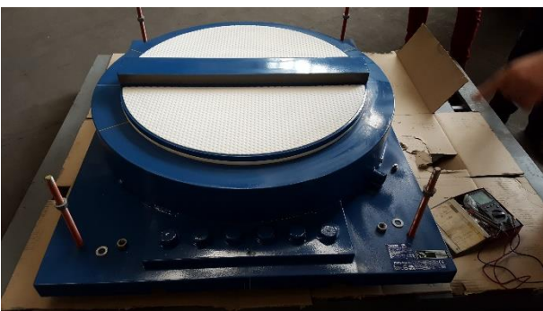
Figure 15. The piston of this guided-sliding pot bearing has a guide bar along the longitudinal axis for resisting transverse movements
