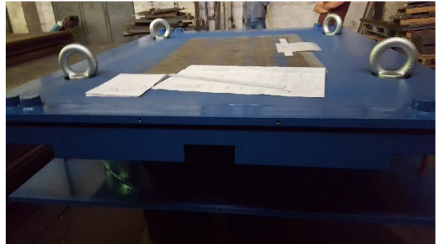
Figure 16. Guided-sliding pot bearing following placing of sliding plate on top of piston, with recess in sliding plate for the piston's guide bar
