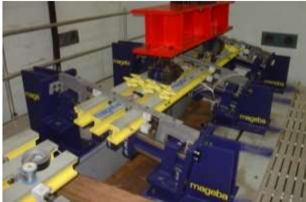
Figure 8. Fatigue testing of Tensa-Modular joint – one specimen.
