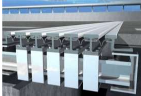
Figure 2. Representation of an installed Tensa-Modular expansion joint (cross section at a support bar), showing stirrup connections to centerbeams.
