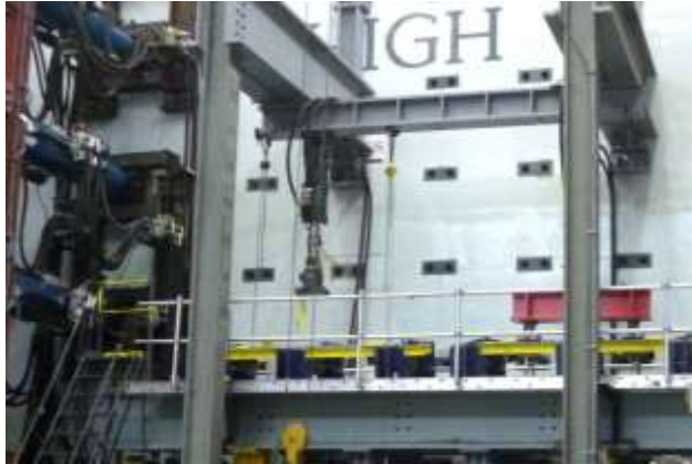
Figure 7. Fatigue testing of Tensa-Modular joint – testing rig at ATLSS / Lehigh University.
