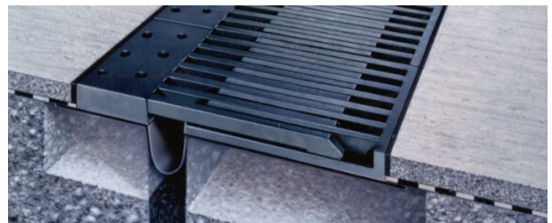
Figure 4. The Tensa-Flex sliding finger joint is fabricated from steel and rubber, with the finger plates pre-stressed downwards to remain in contact with the supporting surface at all times
