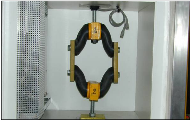
Fig. 3: Testing of Mageba's 4 th generation control springs at -20°C
