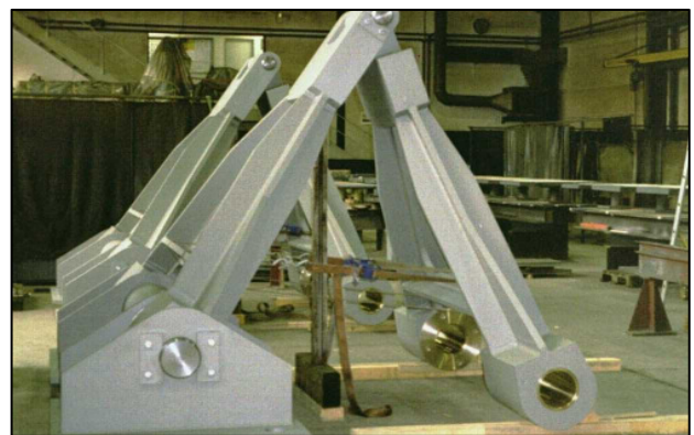
Fig. 13: A wind shoe for the Irtysh River Bridge - during assembly
