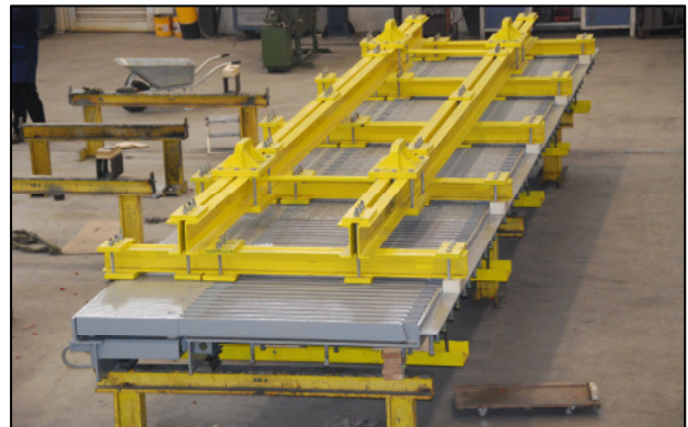
Fig. 9: A sliding finger joint for the Audubon Bridge USA (with transportation frame on top)
