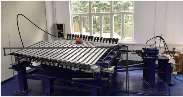
Figure 5. Opening Movement and Vibration (OMV) Test per NCHRP Report 467
