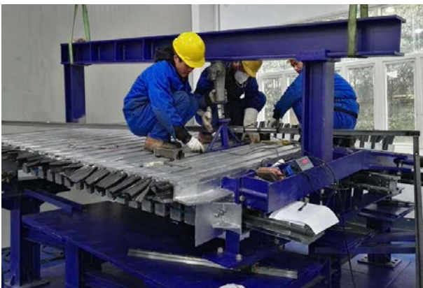
Figure 6. Seal Push-Out (SPO) test in accordance with NCHRP Report 467
