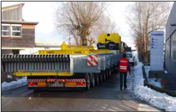
Fig. 14: Road transport from the factory in Austria of a joint for the Incheon Bridge
