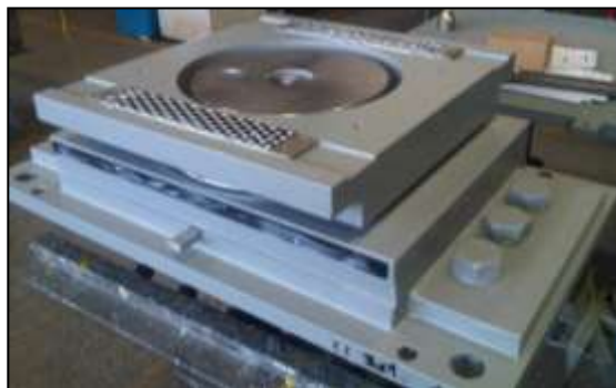
Figure 22. A guided sliding uplift bearing (allowing longitudinal movements, resisting transverse forces), during assembly (before placing of sliding plate on top or guide bars at each side).
