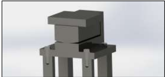
Figure 13. Section of bearing shown in Figure 12. The curved lower surface of the upper element has shear key connections to the plate below (as shown in Figure 15), allowing it to rotate but not to move.
