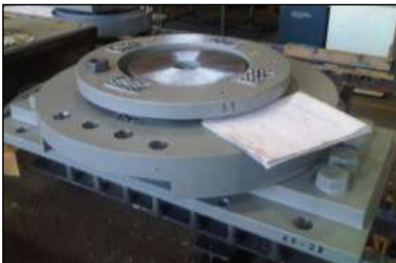
Figure 24. A fixed uplift bearing during assembly (before placing of top plate).
