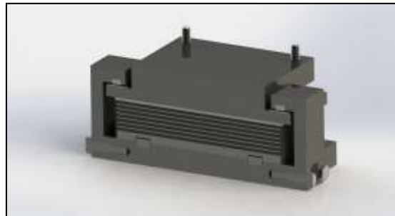
Figure 7. Section through the free sliding uplift bearing. The elastomeric pad is held in place by keys in the steel plate at its base, and the bearing's upper plate can slide across its PTFE top surface.
