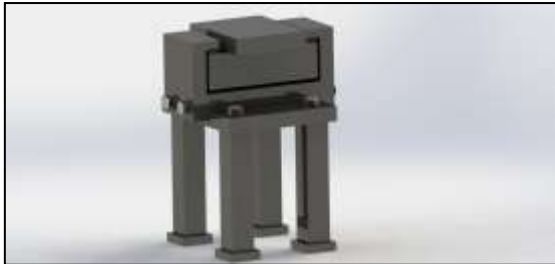
Figure 12. Rendering of a fixed linear rocker bearing with uplift protection clamps at each side. The bearings feature anchor sockets for connection to a concrete support structure beneath.
