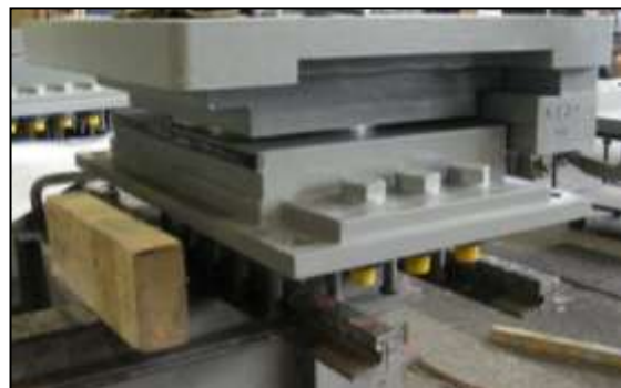
Figure 23. The guided sliding uplift bearing shown in Figure 22, following placing of the sliding plate on top but before fixing of the guide bar at one side.
