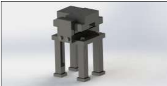
Figure 14. Rendering of a guided sliding linear rocker bearing with uplift protection clamps at each side.
