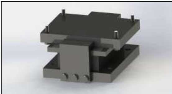
Figure 6. Design of the free sliding uplift bearing, with a reinforced elastomeric pad at its core. The uplift clamps (bolted) at each side resist uplift but allow limited transverse sliding movement.
