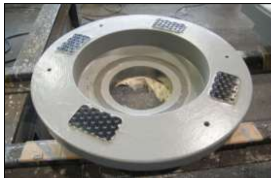
Figure 25. The main uplift-resisting element of the fixed uplift bearing shown in Figure 24.
