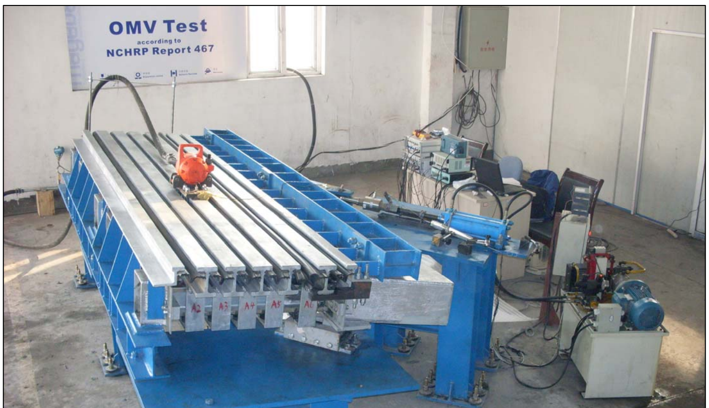
Figure 7. Opening Movement & Vibration (OMV) Test
