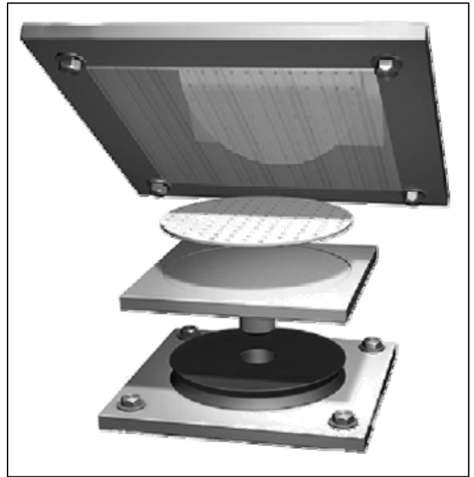
Figure 3. Typical configuration of a multi-directional Disc Bearing
