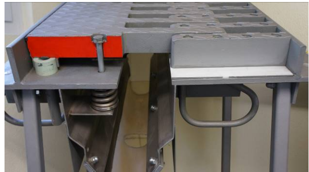
Figure 20. Full-scale model of Tensa®Finger (Type GF) sliding finger joint, showing its construction
