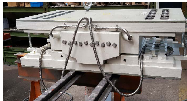
Figure 7. Bearing for fixed end of one bridge, with stainless steel conduits for cables to sensors
