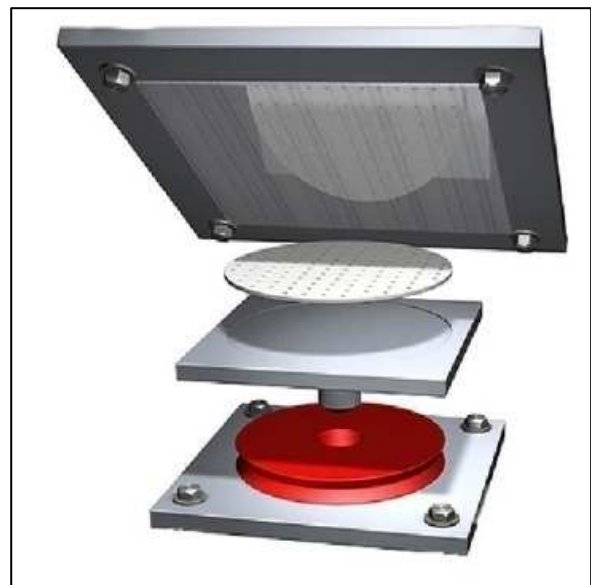
Fig. 8-The structure of a typical disk bearing
