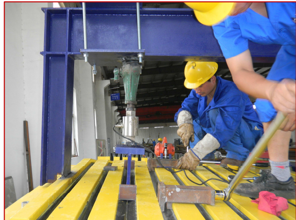
Fig. 7-Seal Push Out (SPO) test
