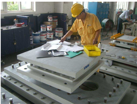
Fig. 9-Quality control during the production of a disk bearing
