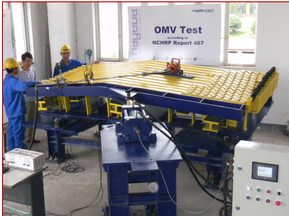
Fig. 6-Opening Movement & Vibration (OMV) test of an 11-gap modular joint
